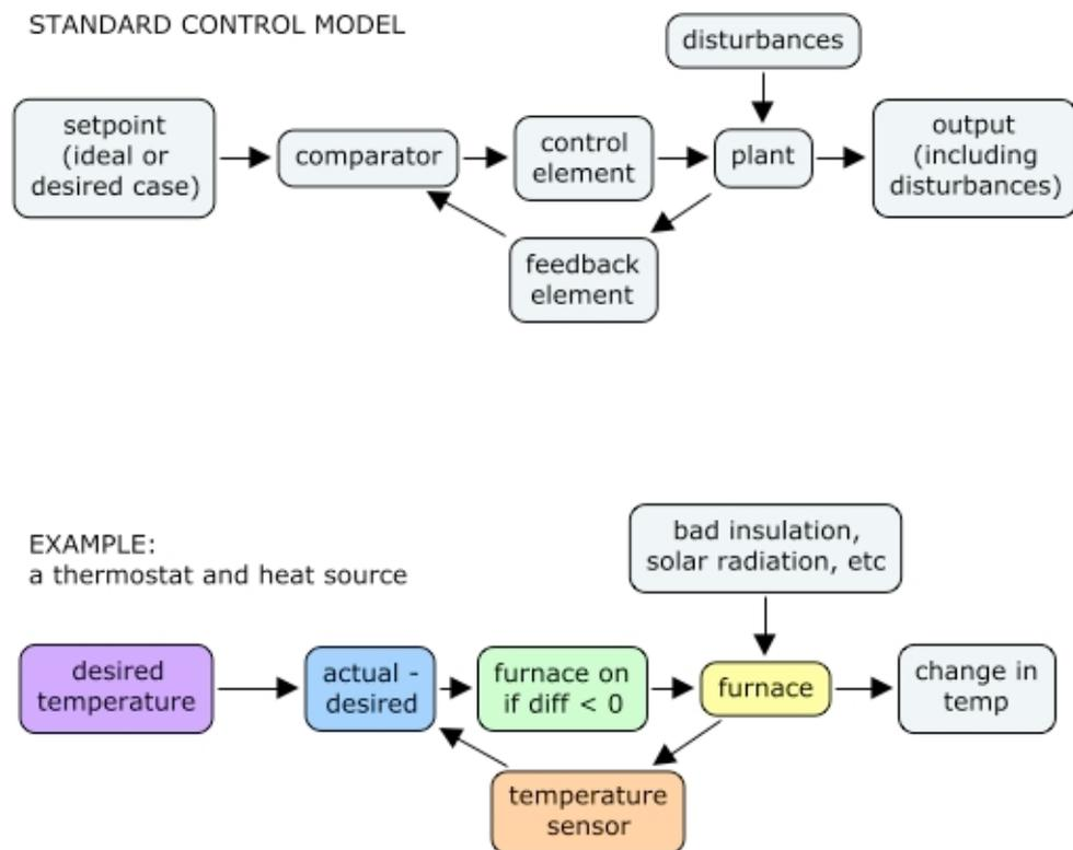
Figure 2: A typical block diagram for a control system with a feedback loop, and example.
