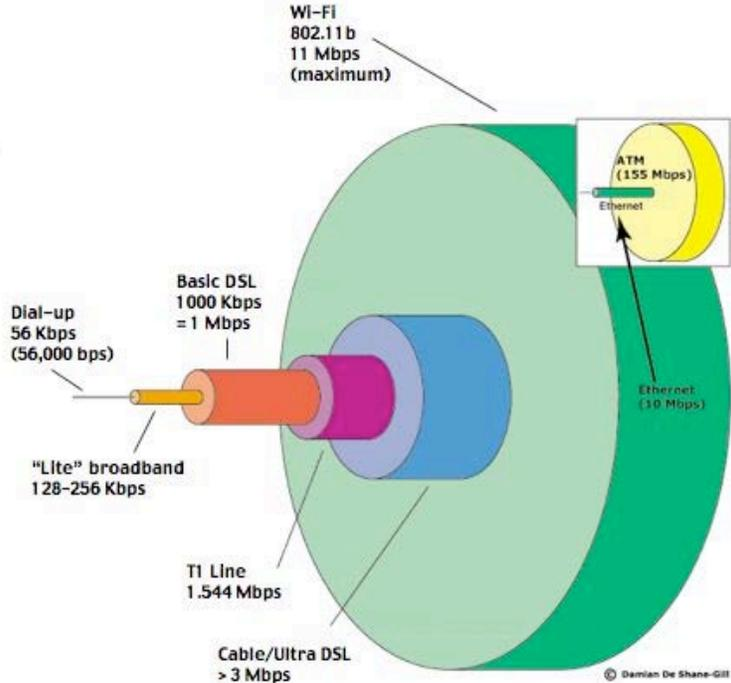
Figure 2 provides a schematic representation of the speeds provided by various access
